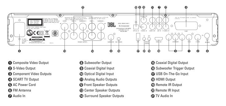
**O** Composite Video Output: Connect this jack to the video input on a television or video projector.
